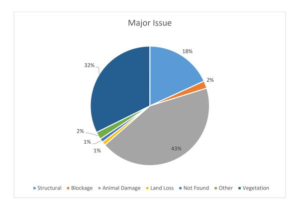
The above graph shows the percentage breakdown of defect type. Animal damage on the stopbanks is the largest of the major defects at 43%, followed by vegetation at 32%.
