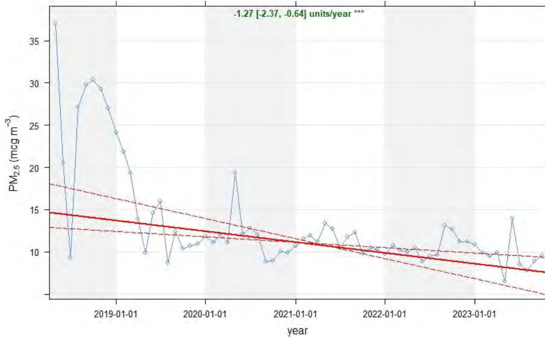
Figure 1: TheilSen 5-year trend plot using monthly PM_{2.5} concentrations for Invercargill (2019-2023 inclusive). Trend is indicated by the solid red line, with the confidence intervals identified using dotted line.
