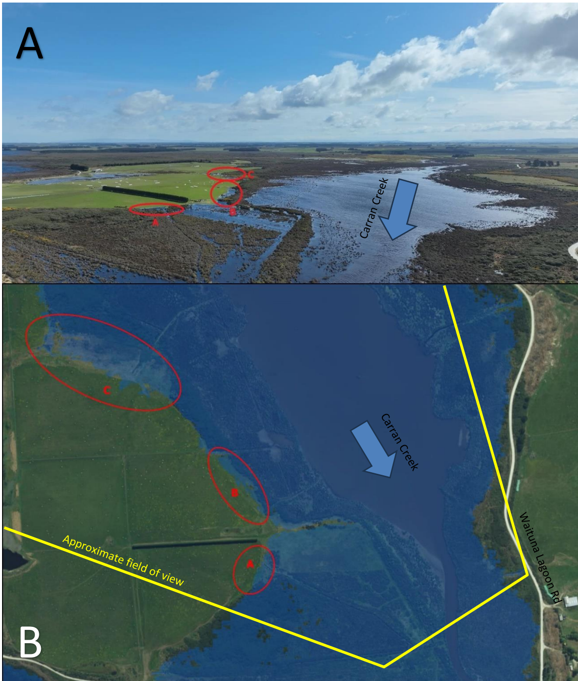
Figure 2: Panel A: Carran Creek right bank above Waghorn Road bridge on 23 September 2024 when lagoon level was 2.59 m; Panel B: model results for lagoon level at 2.5 m (modelled inundation extent is the same for all simulated river flows and channel vegetation conditions at this location when lagoon levels are 2.5 m).
