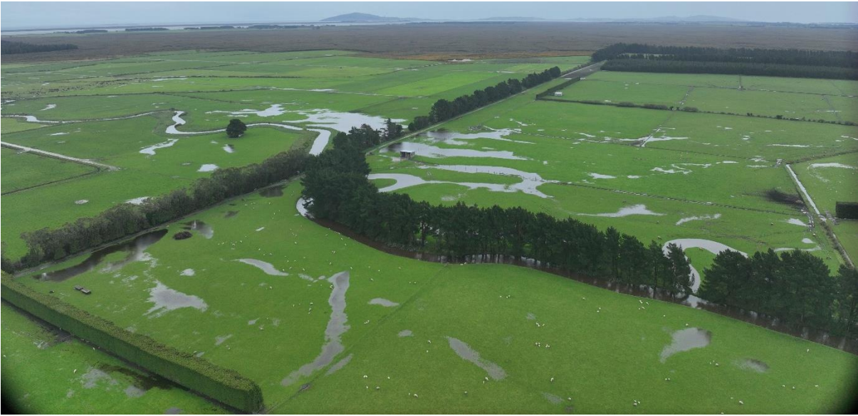
Figure 8: Waituna Creek on 24 October 2024, looking downstream from Marshall Road, North of intersection with Hanson Road. Lagoon open, lagoon water level approximately 0.7 m, creek flow very high (greater than 90 th percentile). The upstream end of the Waituna Creek Model coincides with the right margin of the aerial photo. The model shows no inundation in this reach.
