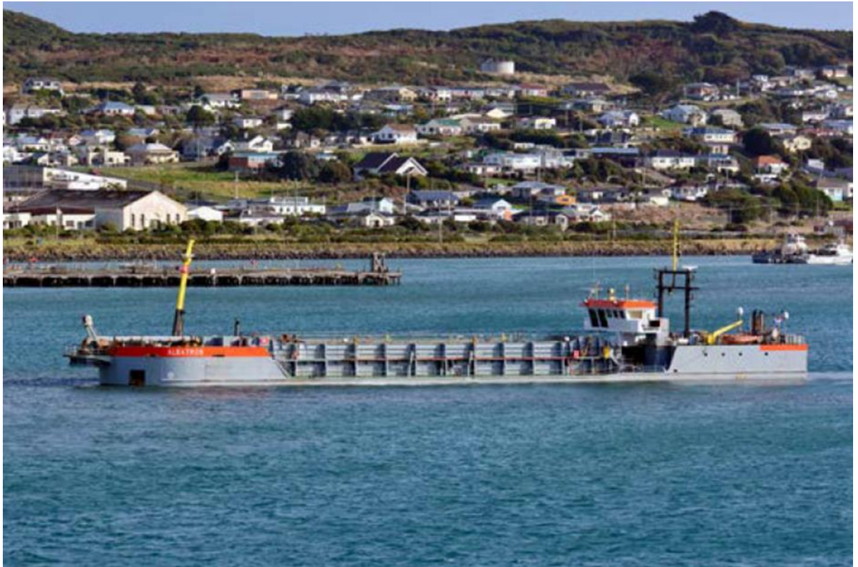
Figure 16: Trailer Hopper Suction Dredge
