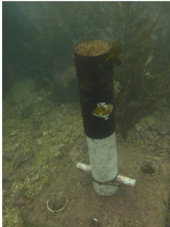
Figure A4-2. Underwater image of one of the acoustic monitoring stations in the Bluff Port Area. The acoustic recorder sits within the PVC pipe and the mesh covering reduces biofouling and potential flow noise.
