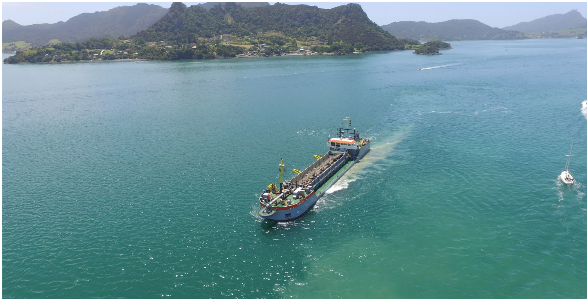
Figure 15: Sediment plume effect from dredging / sediment or rock deposition to sea (indicative only)
