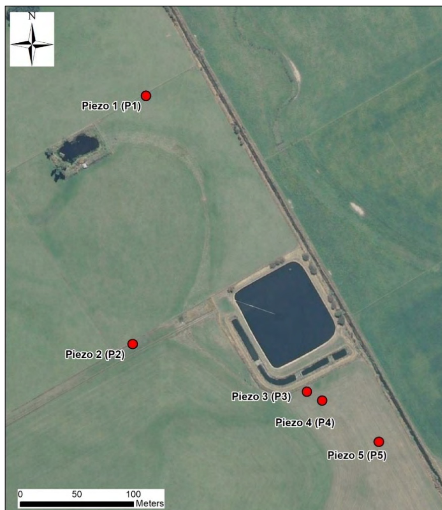
Figure 3.5: Location of SDC groundwater quality monitoring piezometers at the Riversdale WWTP.
