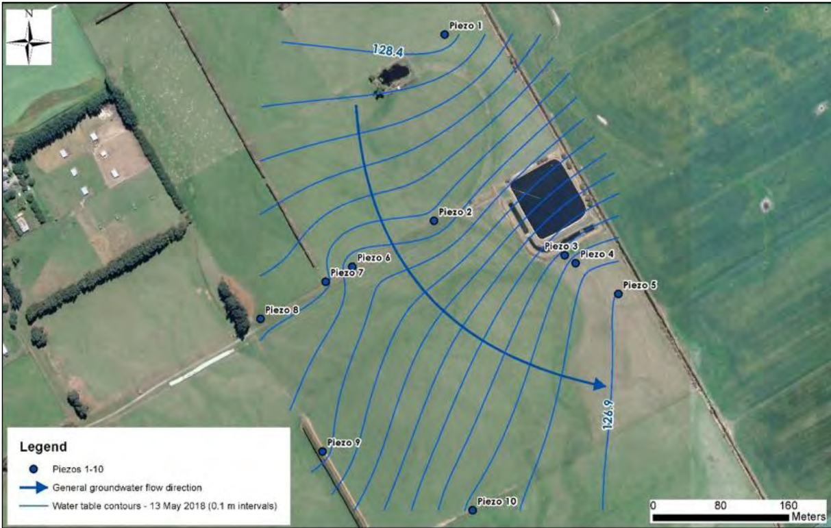
Figure 3.10: Location of groundwater monitoring piezometers at the Riversdale WWTP and inferred groundwater flow direction based on data up to May, 2018 (Dommissie, 2019)
