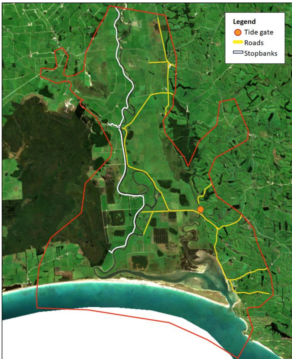
Figure 3-1: Locations of the tide gate, roads and stopbanks within the model extent (red outline).
