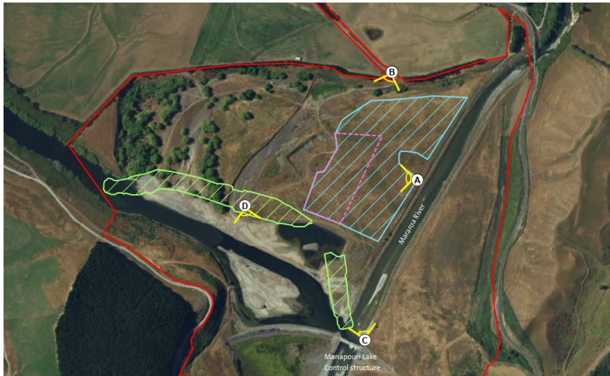
Figure 5.6: Spoil disposal area (blue outline), gravel stockpile cell (pink outline). (Source: Appendix H).
