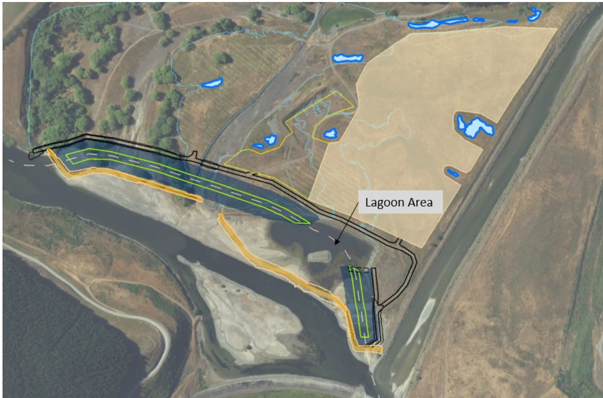
Figure 5.2: Stage 2 – Excavation area shown in partly transparent dark blue; base of channel shown with green outline.
