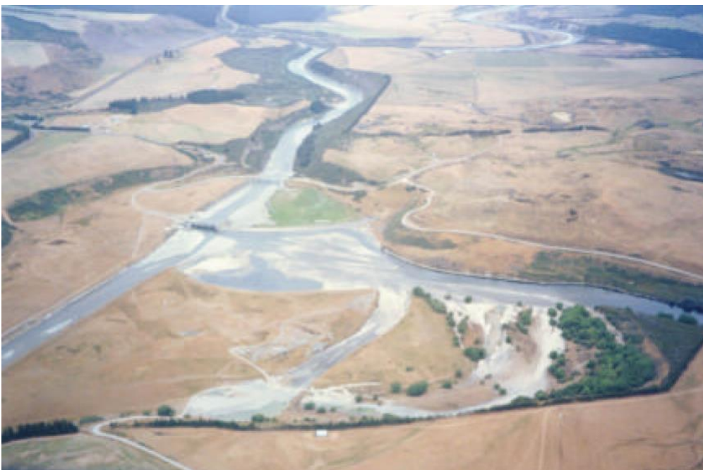
Figure 2.3: MLC looking south, January 1999. The Waiau Arm enters from the right, the Mararoa diversion cut flows from the lower left. The original confluence is on the right of the photo with the channel in the lower middle understood to be a diversion excavated during construction of MLC.
