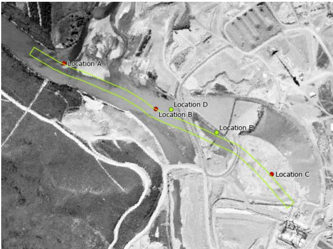
Figure 5.5: Trial hole locations and anticipated in-stream channel excavation footprint, overlaid on aerial image from MLC construction, March 1974
