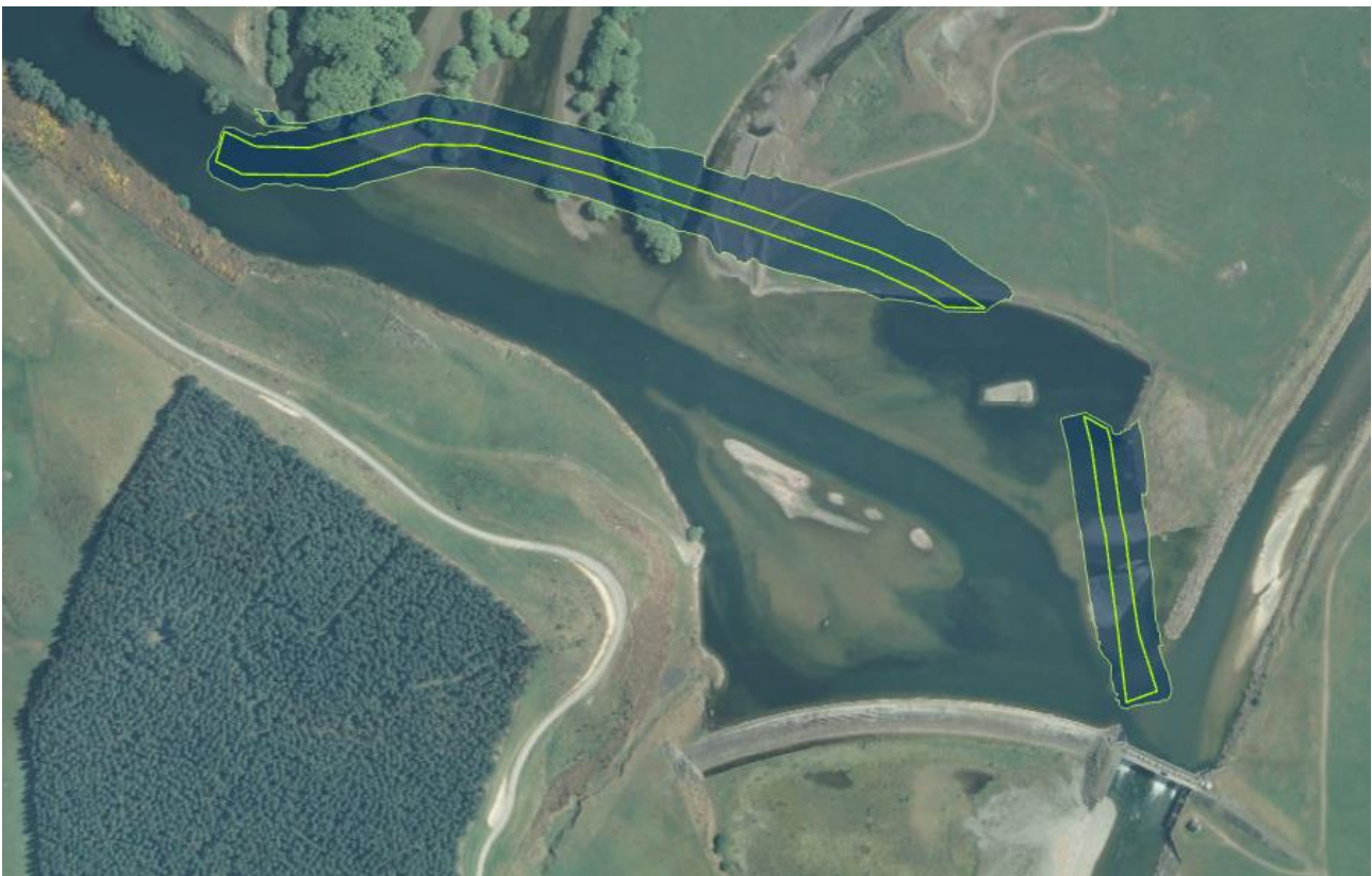
Figure 6.1: Proposed 'parallel channel' excavation arrangement - trapezoidal channel with base at RL 172.0 m, excavation extent in dark blue shading.
