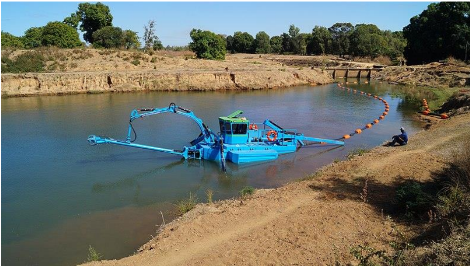
Figure A.1: Cutter suction dredge
