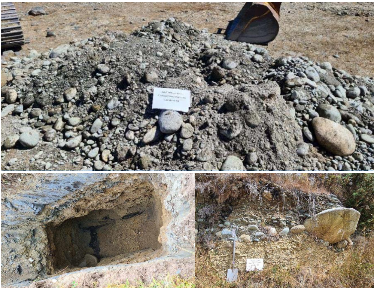
Figure 5.1: Alluvial gravels from left bank test pits (top); Clayey-silt in right bank test pits (bottom left); glacial till observed on right bank, including large-sized boulders (bottom right).
