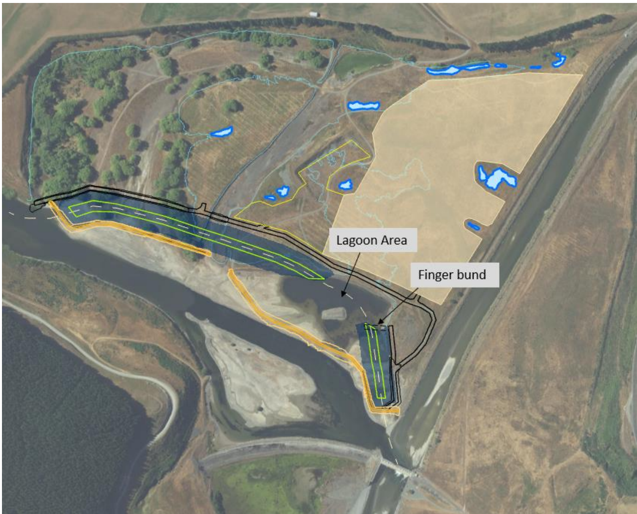
Figure 6.6: Excavation Stage 2, with channel base at RL 172 shown in green outline, and excavation area shown in blue. Dashed ‘finger-bund’ shown to allow excavation within lagoon area.
