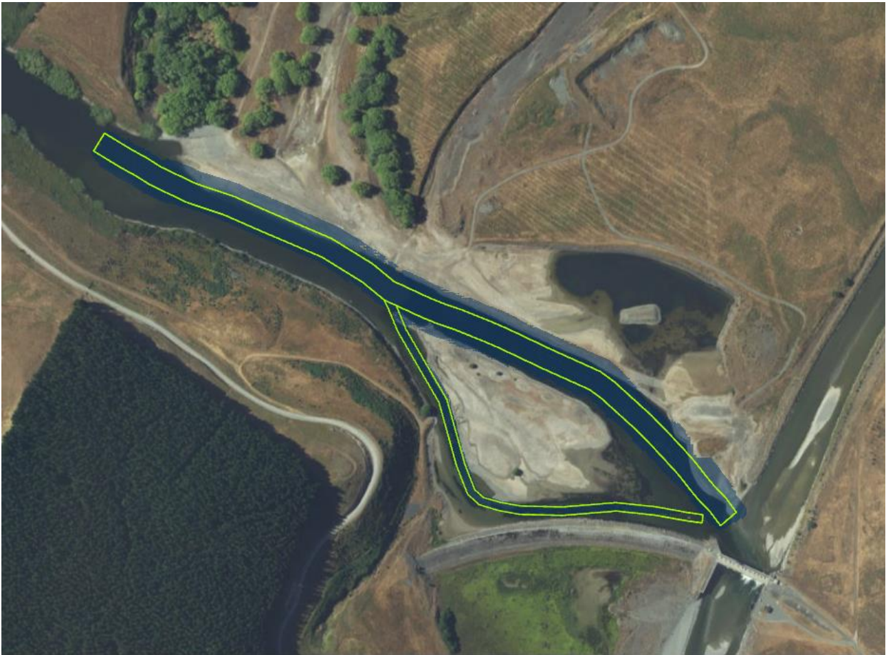
Figure A.9: In-channel excavation arrangement developed - trapezoidal channel with base at RL 172.0 m (main channel) and RL 175.25 m (southern channel), excavation extent in dark blue shading.
