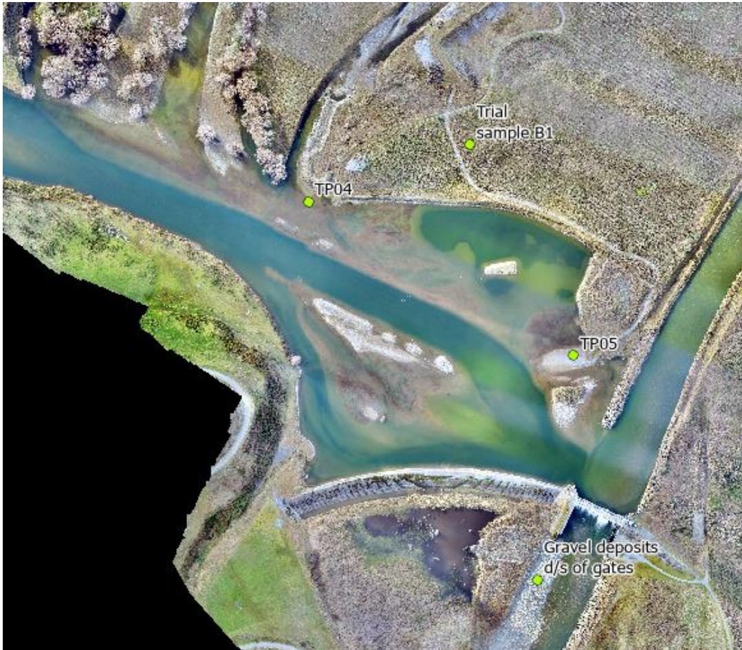
Figure 5.6: Potential gravel sources which have been investigated.
