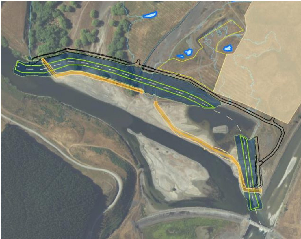
Figure 6.3: Proposed excavation arrangement, with excavated channel footprint shown blue with channel base in green outline, haul roads in black outline, bunds to isolate the works from the Waiau Arm in orange.
