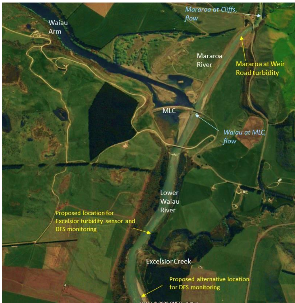
Figure 3-3: Locations of turbidity and flow recorders to be used in the monitoring programme over the duration of the Project.
