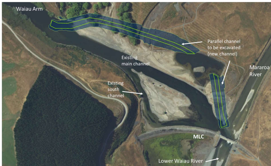
Figure 1-1: Configuration of the channels following the proposed excavation. The main and south channels currently convey all water from the Waiau Arm to the MLC. After excavation of the new channel, the main and south channels will continue to convey smaller proportions of the flow than at present. Refer to text below for more detail.
