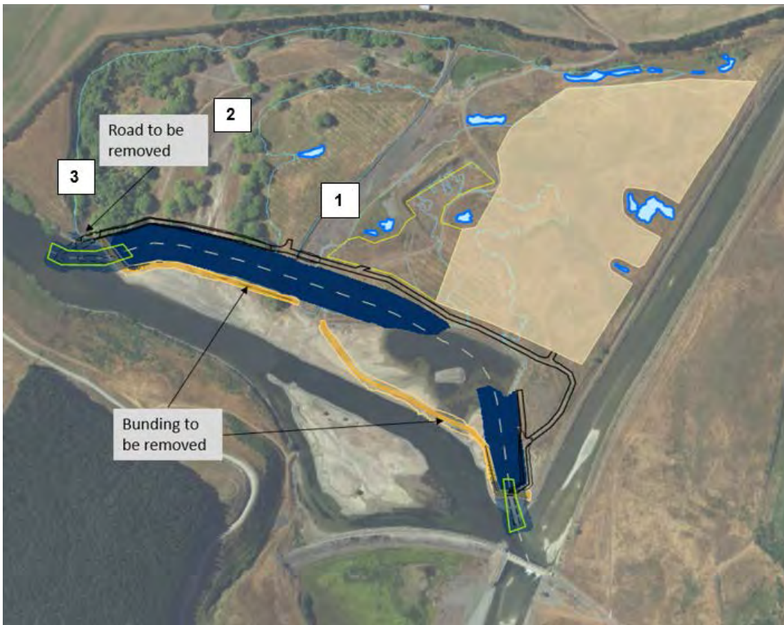
Figure 5. Excavation of the new channel (dark blue) and the inlet and outlet (light blue with green) tying in with Waiau Arm, construction bunds (orange), and permanent haul road (black). Dashed black lines indicate temporary (construction only) haul roads (from Damwatch, 2023). Channels within the Project site are labelled 1, 2 and 3.
