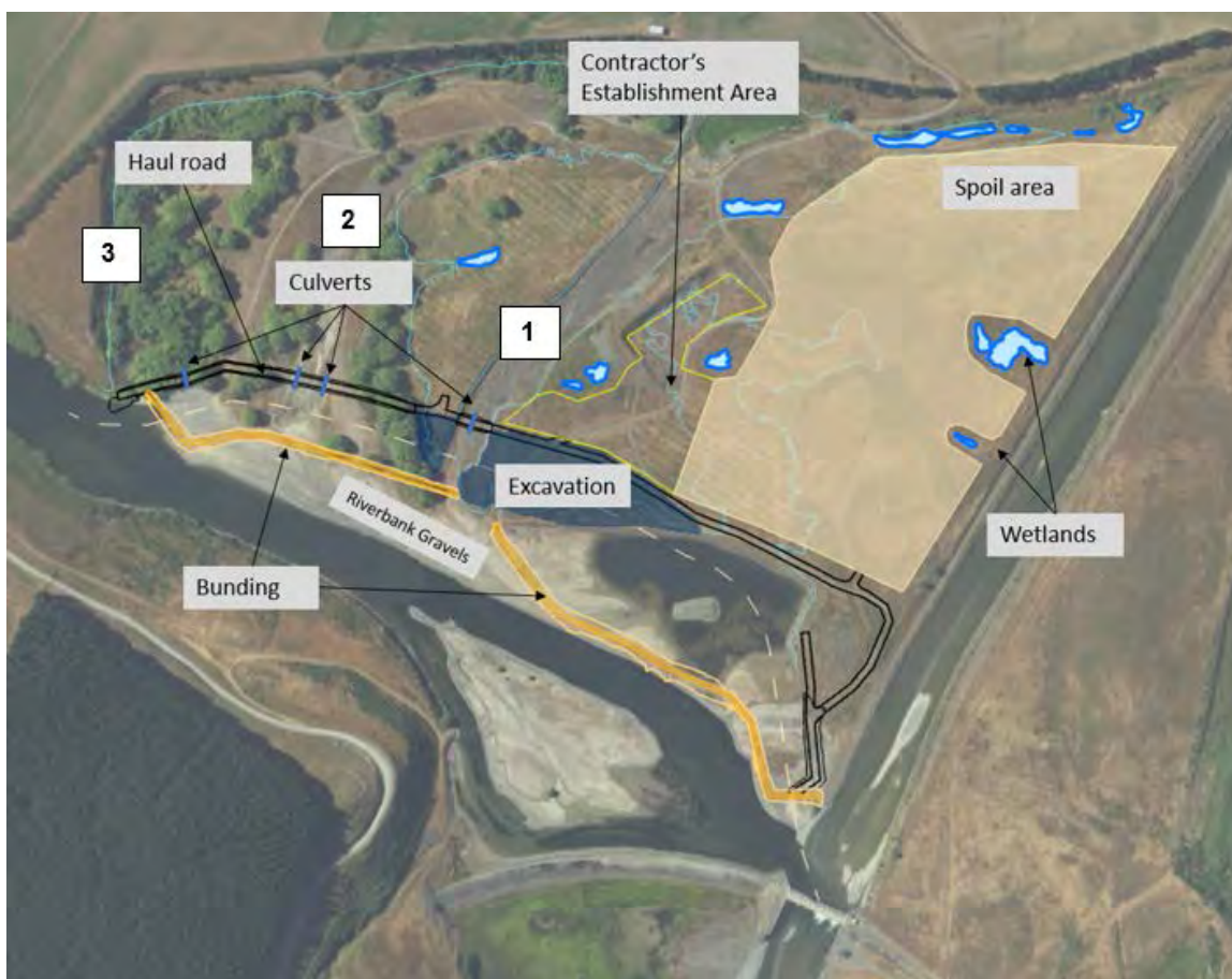
Figure 4. A haul road (black) and bund (orange) are first established to manage sedimentation effects during excavation of the new channel. Culverts will be installed in Channels 1 & 2 but not in Channel 3. Channels within the Project site are labelled 1, 2 and 3.
