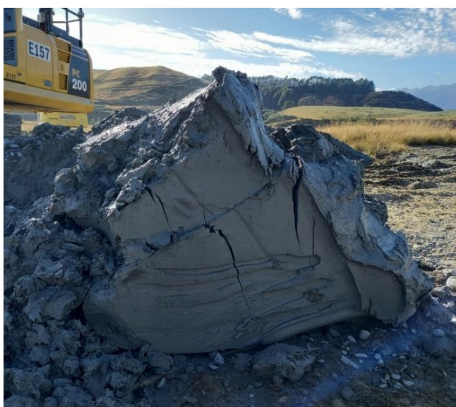
Figure 2: Clay material excavated from Waiau Arm in 2023 trial excavation
