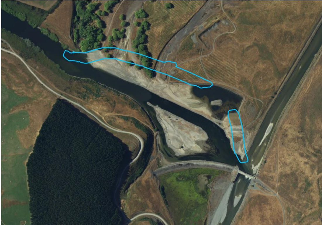
Figure 1: Proposed channel excavation alignment
