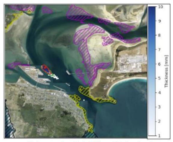
Worst-case sediment footprint (from a P3 release location over a spring tide cycle from 1 h before to 4 h after high water) with seabed resuspension excluded. The green and red contours highlight 2 and 4 mm respectively. The purple, yellow and black hatched patch represents the seagrass, rocky and mataital area respectively. Deposition thickness of less than 1mm were masked (from Zyngfogel & McComb, 2023).
