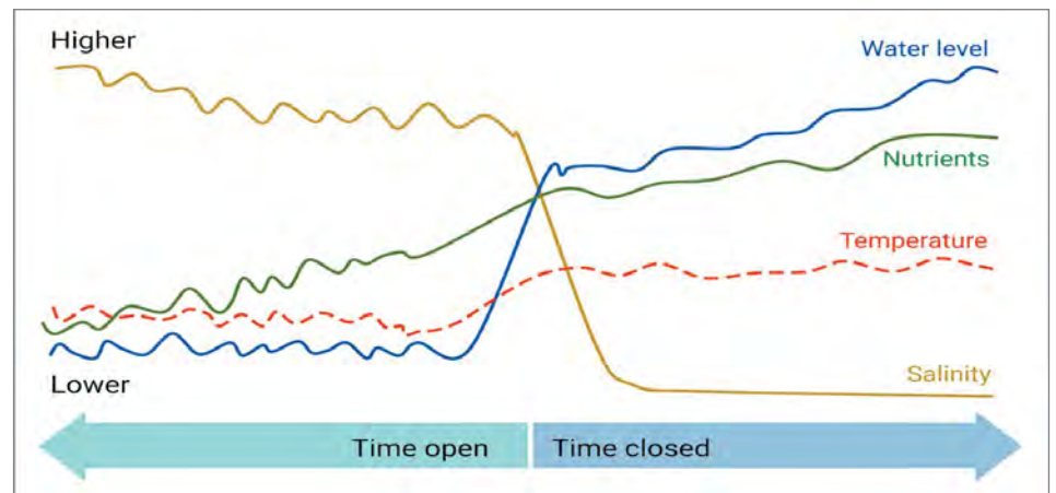
Figure 2: Key changes in the waters of Waituna Lagoon with time after opening or closing to the sea.
