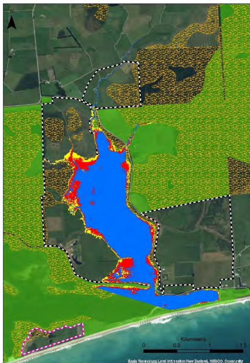
Figure 13. Extent of inundated land from Waituna creek (top left), Moffat Creek (top right) and Carran Creek (bottom) at different lagoon levels, modelled under a scenario of mean flow and channel vegetated. Purchased properties outlined in black/white, land not purchased outlined in pink/white. Walsh et al 2016.
